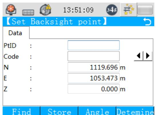
**A: (enter station coordinate and backsight point coordinate to set the backsight orientation angle)**
