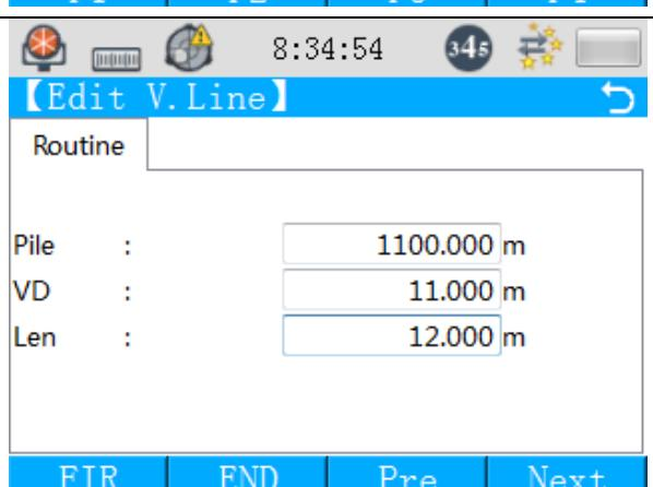
The alignment data can be processed with this menu and the operations are the same as that for editing horizontal alignment data. See “6.11.1.2 Edit horizontal alignment”.
