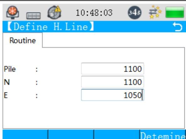
With detailed data of start point entered, press “F4” (Determine) to enter main line input process screen:
