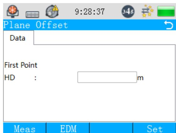
⑤ Sight prism P1 and press “F1” (Meas) to start measuring. (If continuous measurement is adopted, “F4” (Set) shall be pressed when measurement is finished.)
