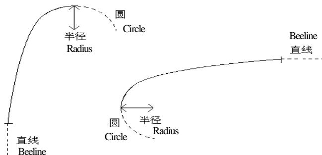
Press the button CUR in main line input process screen and you can define the curve which comprises the minimum radius and arc length. The definition of positive and negative radius is the same as the arc. Similarly, its arc length shall not be negative.
