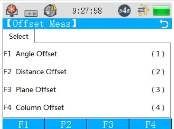
④ Press “F1” or (1) to enter angle offset measurement selection interface.
