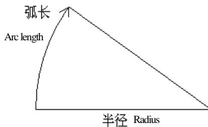
Press the button ARC in main line input process screen and you can define the arc which consists of radius and arc length. Radius is defined as moving direction along the arc. The radius is positive when it turns right and negative when it turns left. The arc length shall not be negative.
