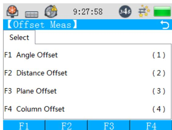
④ Press “F3” or (3) to enter plane offset measurement interface.
