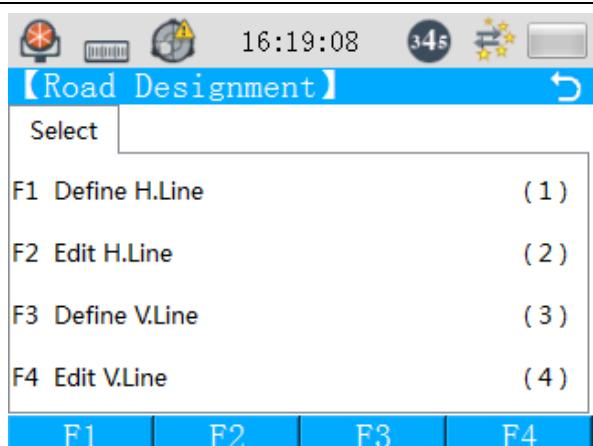
② Press “F1” or (1) to enter horizontal alignment start point input interface from road designment menu.
