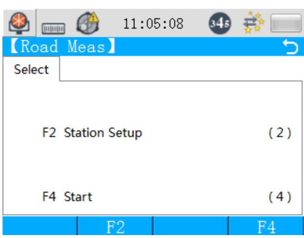
② To set station coordinates and azimuth, press “F2” or (2) to enter station setup interface.
