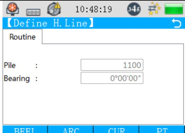
The horizontal alignment system provides four definition functions: beeline, arc, curve and point. Press one of the four function keys, enter details of the pile number and elements of alignment will be generated. Press “F4” (Determine) and the system software will calculate the new pile number and bearing and return to the main alignment screen; then, you can define another line type. New alignment elements can only be added to end portion of the original alignment file.
