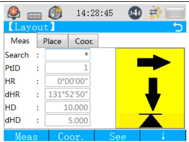
Method 2: Press “F2” (stake) to enter a layout point without point name and the need to store its data.
