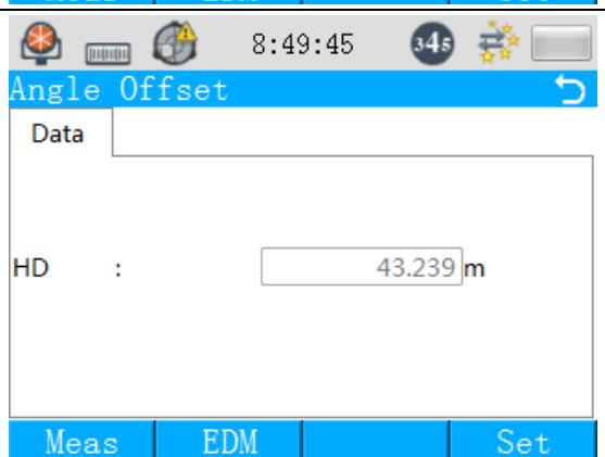
⑦ Sight target point A0 with horizontal clamp screw and tangent. Press “F4” (Set) to display elevation difference, horizontal distance and slope difference between instrument and A0 as well as coordinates of target point (N, E, Z).
